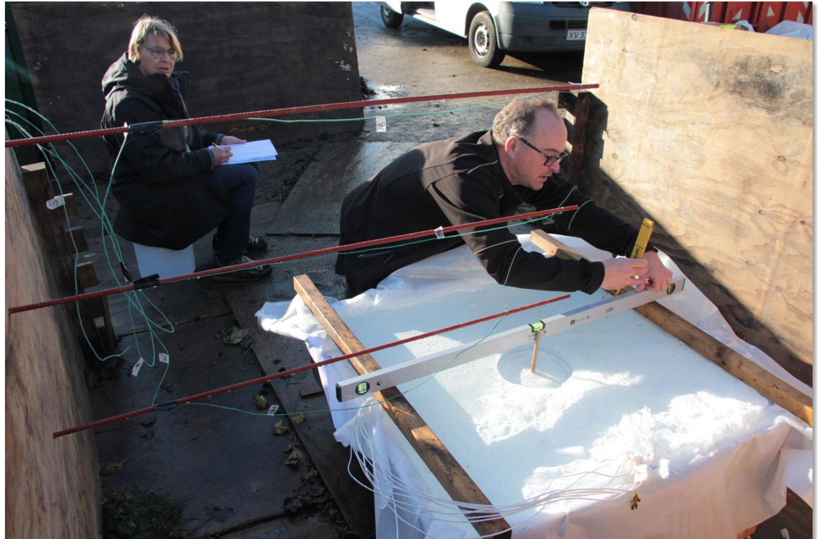
Measurement of two surface profiles each before and after the burn
